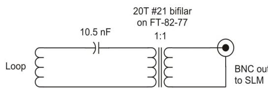
10 turns of wire. The measured impedance was  $0.9 + j111$  ohms at 137 kHz. To avoid dropping the voltage across that 111 ohms of reactance, the loop would have to be fed into a receiver input impedance of 10 times (or more) of that value, i.e., 1110 ohms. At the time, I wanted to use the 50 ohm input on the SLM. So I used the circuit below:
