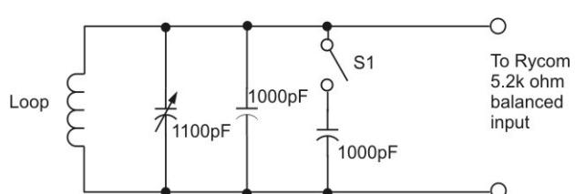
The tuning range is about 125 to 150 kHz with S1 closed, and 145 to 198 kHz with it open. I measured the
