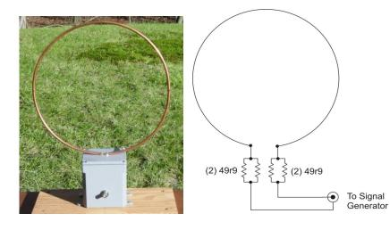
Simple! The idea was to present a 50 ohm load to the generator, and essentially balance the loop by placing 25 ohm resistors in each side. Since the inductance of the loop is quite low at 137 kHz, an impedance bridge measured 50.1 +j0.7 ohms. You could insert a 1 uF film capacitor in series with the circuit and eliminate the inductive reactance if you desire.
