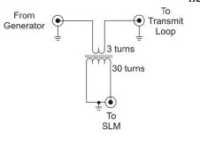
field reading. Here's the schematic of the current transformer:
